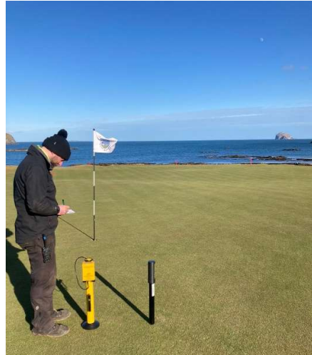
Figure 7: Clegg Hammer and Pogo being used on the 1 st .
