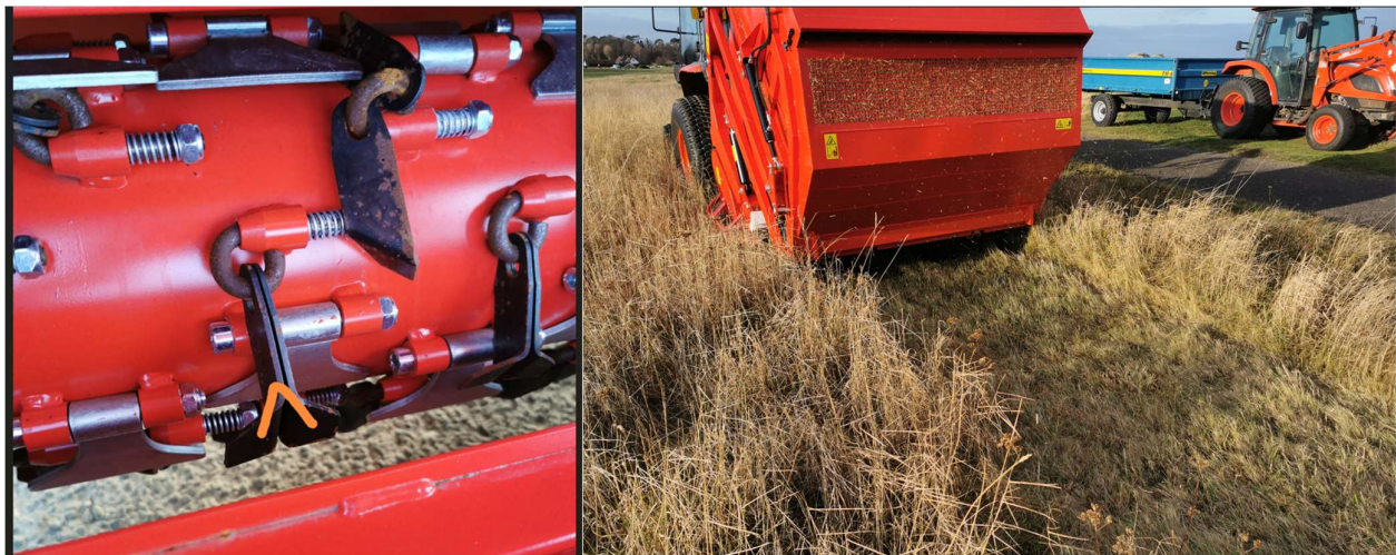
Figure 8: A close up of the flail blades (LHS) and what the rough looks like after being cut (RHS).
