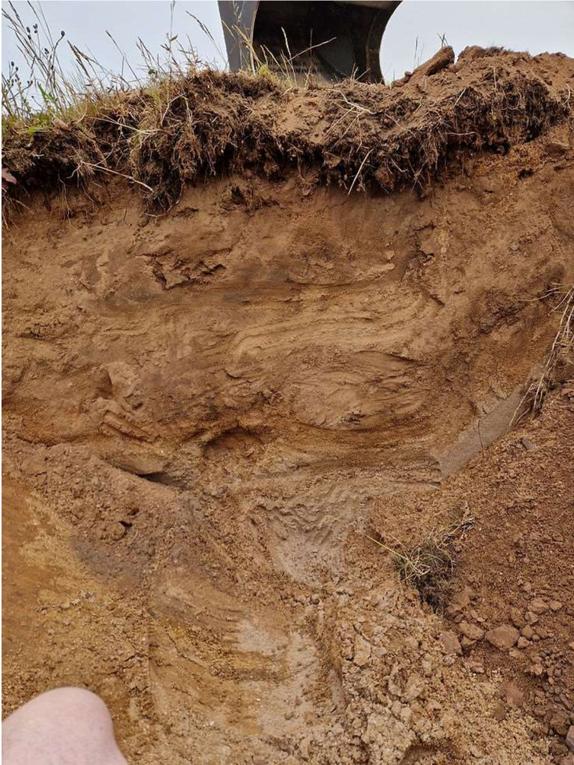
Test hole showing the depth of sand under the existing vegetation.
