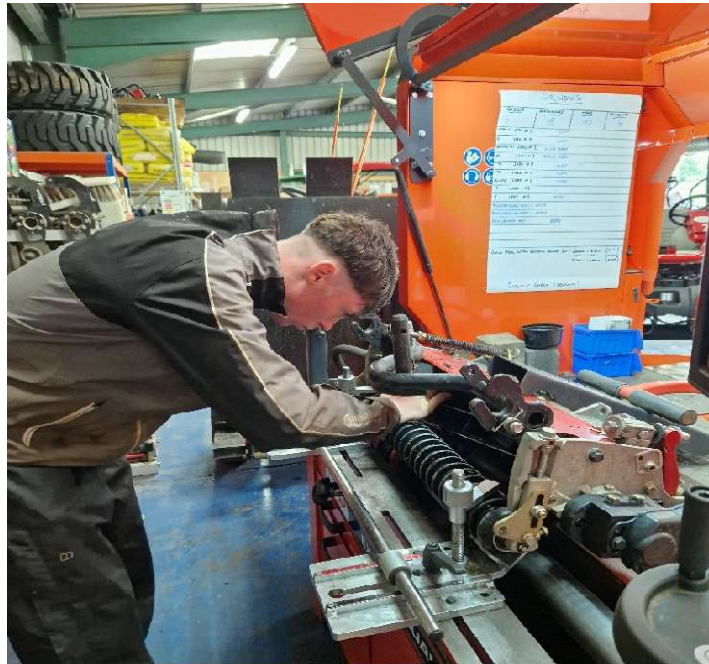
Figure 6: Ryan Yuill getting ready to grind a fairway unit.
