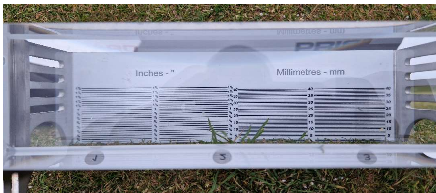
Figure 1 - The Prism Gauge used to show heights of cut showing the different heights the different grass species are currently. Brushing and Grooming will help to reduce this.
