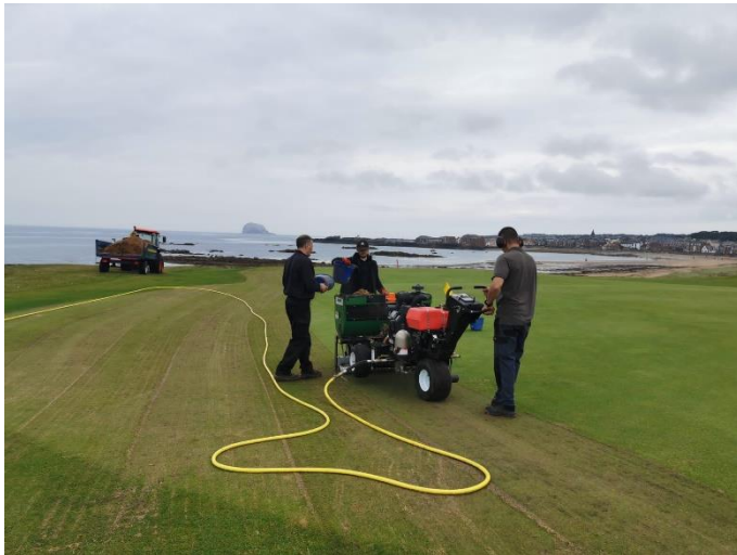
Figure 1. Dryject uses high pressured water to inject the sand into the greens surface.
