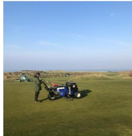
**Guy with our own Air2G2 machine on 5<sup>th</sup> Green injecting compressed air into the root zone.**
